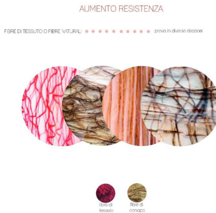
Bioplastics based on agro-food waste, integrating plant fibers and textile waste fibers. Design by Clarita Caliendo; Scientific coordination by Carla Langella; Co-tutor: Carlo Santulli.
