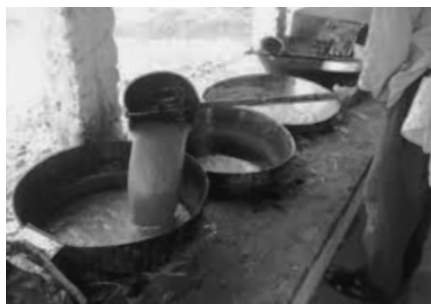
Figure 2.1 The concentration of sugarcane juice prior to crystallization. Source: Leandro Vilar. 7
