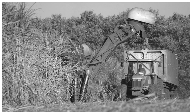
Figure 2.8 Green sugarcane mechanized harvesting in Brazil. Source: Arthur Saraiva, site EMBRAPA. 22
