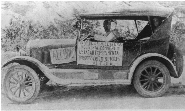
Figure 6.1 One of the first ethanol fuelled vehicles in Brazil, a Ford automobile, specially prepared at the Estação Experimental de Combustíveis e Minérios (today Instituto Nacional de Tecnologia-INT).
