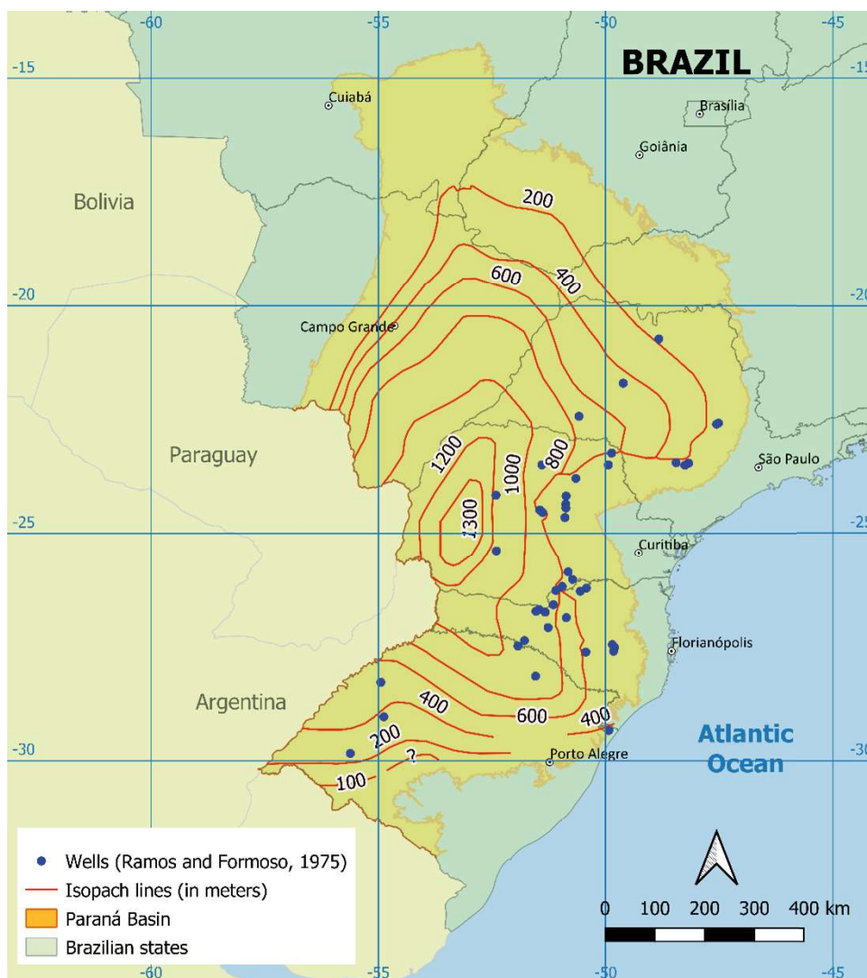
Figure 1 - Isopaque map (in meters) of the Permian section above Irati Formation and the location of the 43 wells analyzed by Ramos & Formoso (1975) in the Paraná Basin (Source: Lima 2021).
