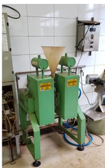
**Figura 3** - *Wet High Intensity Magnetic Separator* (WHIMS)
