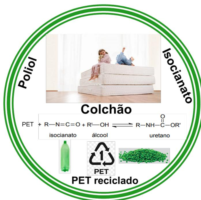
The use of micronized PET as an organic filler in flexible polyurethane foams has both an economic and an ecological appeal, providing a value-added destination for recycled PET. Its even and homogeneous distribution throughout the foam cell structure guarantees the accomplishment of the standard physical properties.
