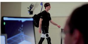
Figura 2: Soft exosuits by Harvard Biodesign Lab.
