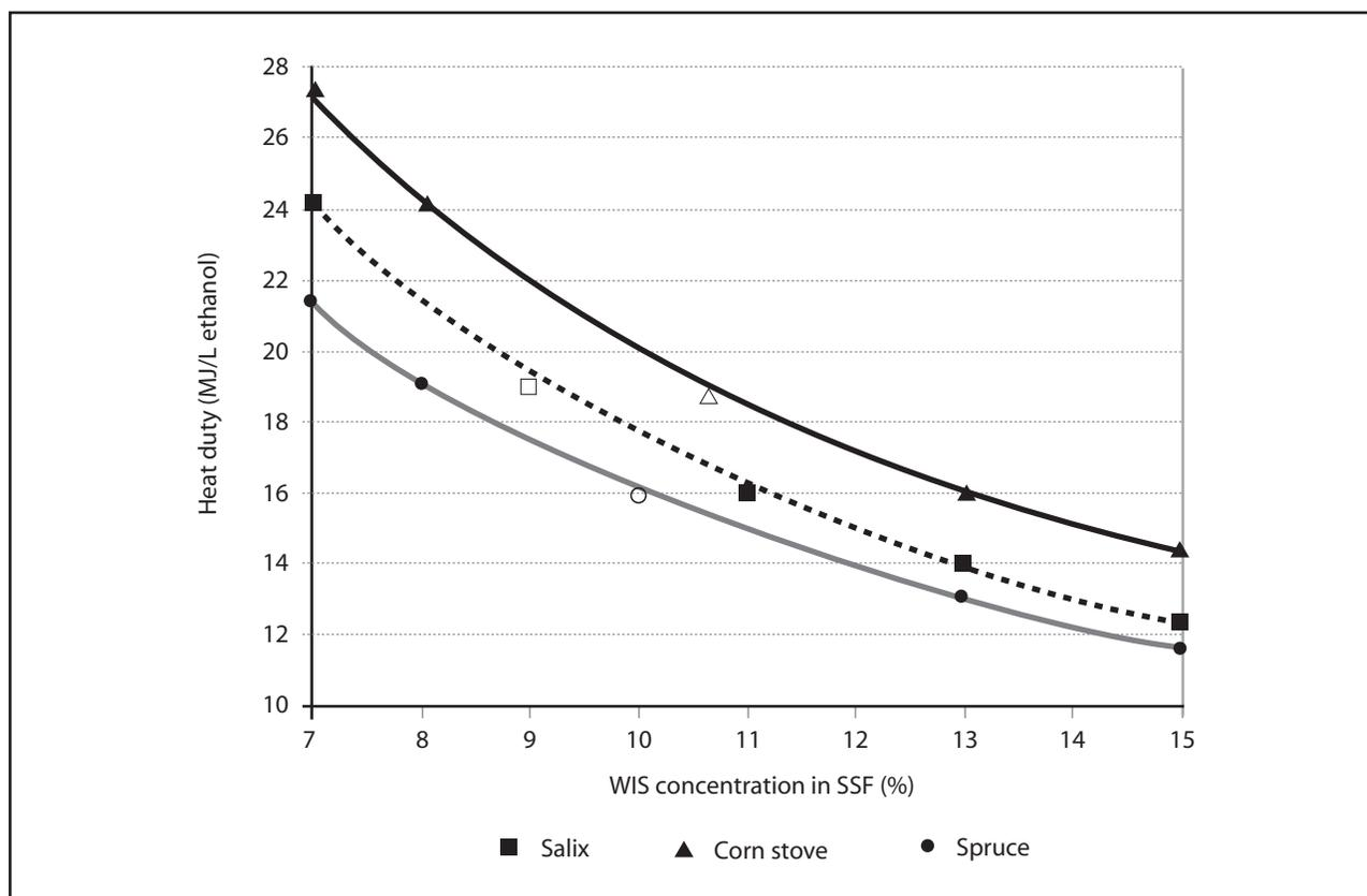
**FIGURE 4** Overall process heat demand as function of WIS concentration in SSF. Ethanol yields are maintained at the same level as in the base cases, which are represented by open symbols. Adapted from reference 59.
