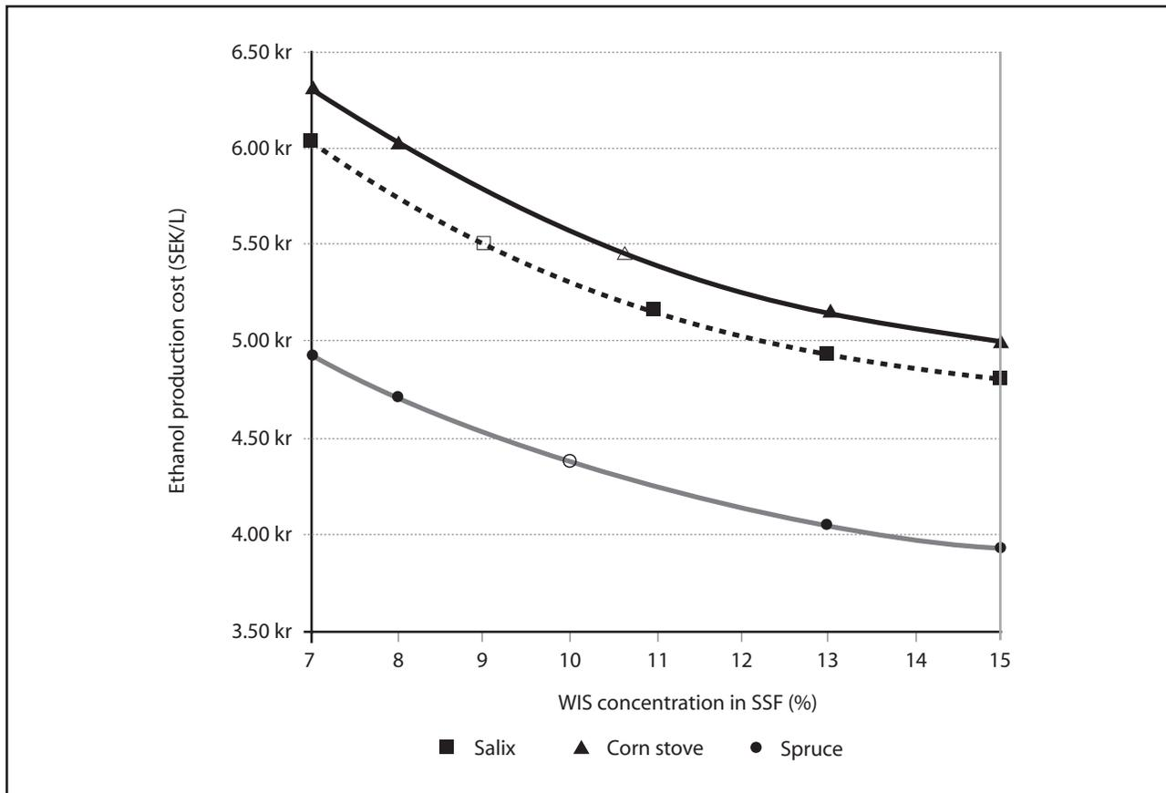
**FIGURE 5** Ethanol production cost as function of the WIS concentration in SSF. Ethanol yields are maintained at the same level as in the base cases, which are represented by open symbols. Adapted from reference 59.
