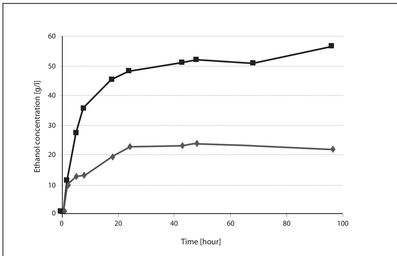
**FIGURE 10** Time course of ethanol concentrations during batch SSF of steam pretreated wheat straw (◆) at 5% WIS and a 50/50 mixture (■) of steam pretreated wheat straw and wheat meal at total WIS of 5%.
