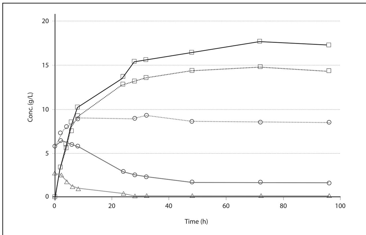
**FIGURE 6** Time course of ethanol ( $\square$ ), glucose ( $\triangle$ ) and xylose ( $\circ$ ) concentration during batch SSF of steam pretreated corn stover at 5% WIS using normal baker's yeast (dotted line) and the genetically modified yeast TMB3400 (solid lines).
