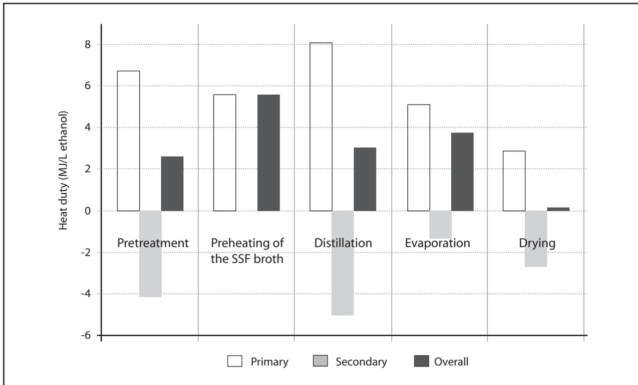
**FIGURE 7** Heat duty of the most energy-demanding process steps in ethanol production from spruce based on steam pretreatment and SSF for a capacity of 200,000 ton spruce (DM) per year. The process is explained more in detail in reference 68. White bars = primary steam demand; grey bars = amount of secondary steam generated; black bars = difference between primary and secondary heat, i.e., the net heat demand for the process. Adapted from reference 69.
