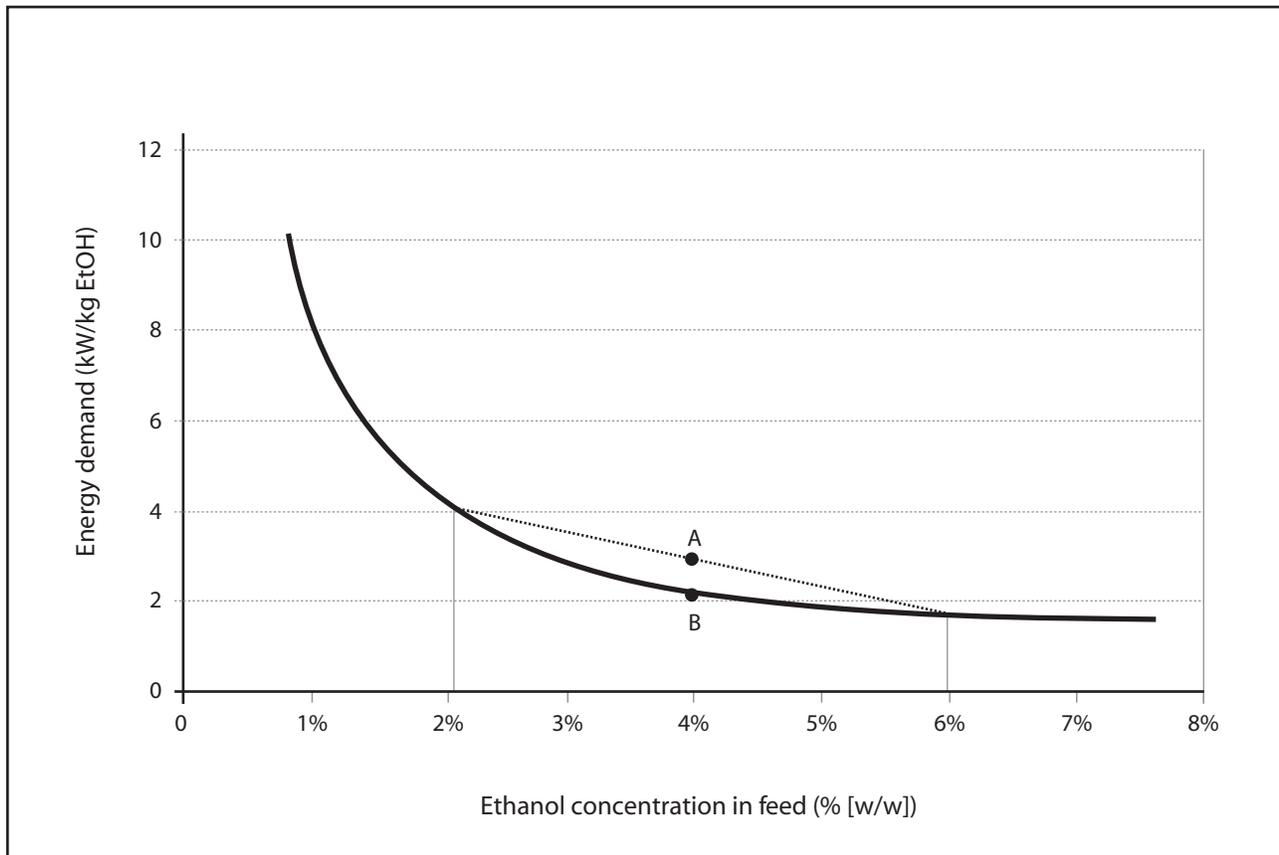
**FIGURE 9** Energy demand in distillation of ethanol to 94 wt-% (see Figure 3). The dotted line shows the energy demand when two streams containing 2 and 6 wt-% ethanol are distilled separately (for instance point A for a 50/50 mixture). This is always higher than the energy demand for distillation for the mixture, which is on the solid line (point B for a 50/50 mixture).
