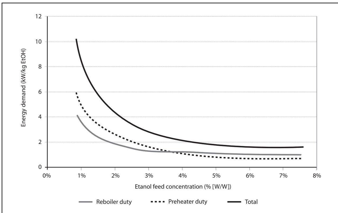
**FIGURE 3** Energy demand in distillation of ethanol to 94 wt% in a distillation unit consisting of two stripper columns and one rectification column connected in series on the vapour side. The set-up is described more in detail in reference 58.
