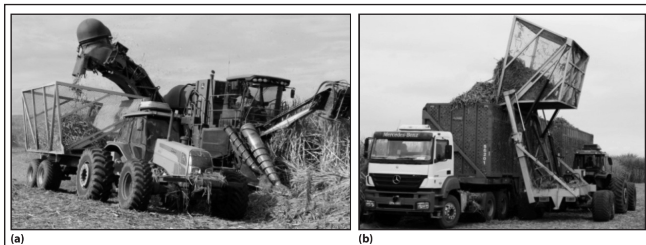
FIGURE 2 (a) Self tipping wagon getting the cane from the harvester; (b) side dumping to the truck.
