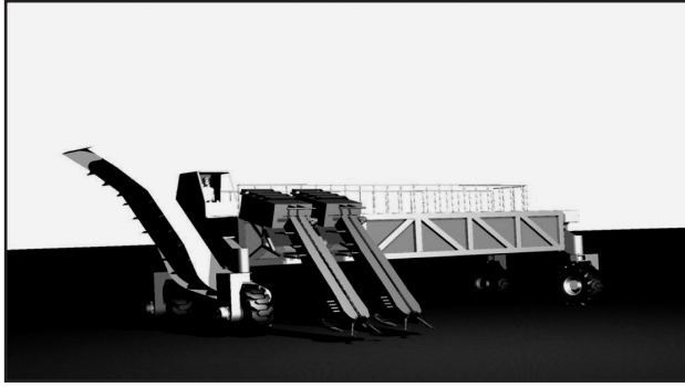
FIGURE 1 Controlled Traffic Structure (ETC) proposed by Bioethanol Science and Technology Laboratory – CTBE – as part of the Low Impact Mechanization (MBI) project for sugarcane production.
