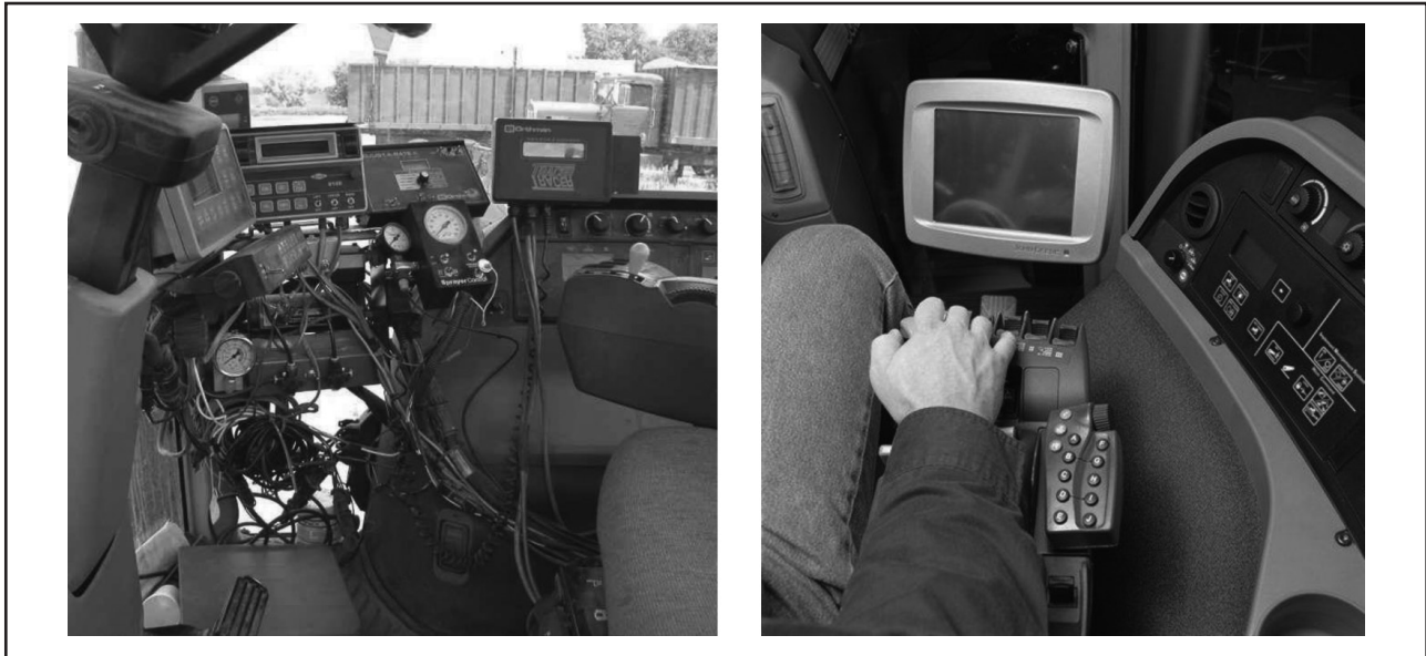
FIGURE 1 Comparative images of a tractor with proprietary solutions – left, and with ISOBUS – right, presented by Hans Jürgen Nissen of John Deere AMS Europe in 2007.
