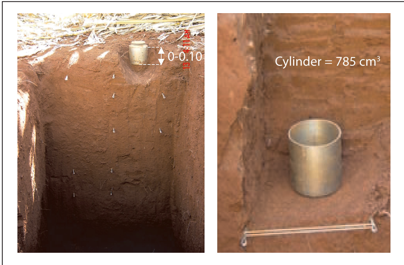
FIGURE 4 Illustration of soil samples collection for analyzing carbon content and determining soil density (cylinders).
