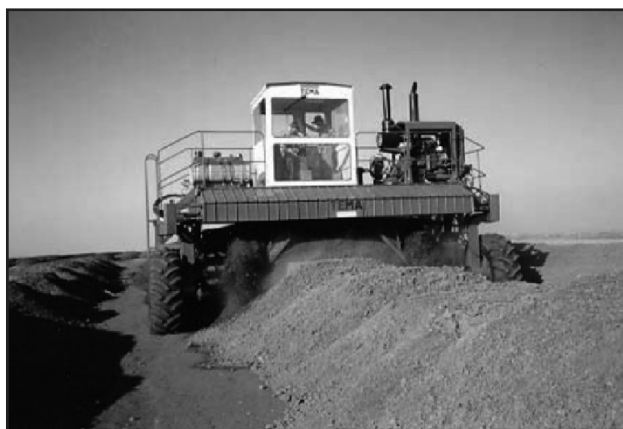
FIGURE 5 Self propelled mixer composting filter cake.
