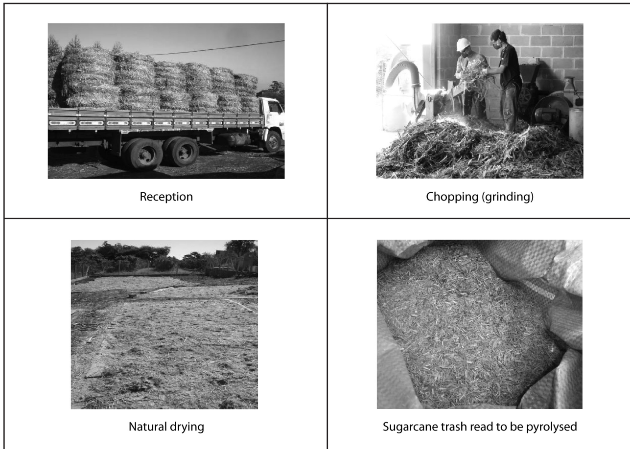
FIGURE 4 Pretreatment phases of sugarcane trash in a biomass fast pyrolysis plant pilot of FEAGRI-UNICAMP.
