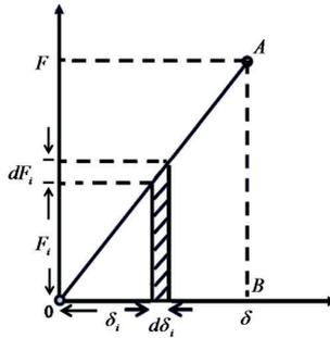
$$W = \int F_i d\delta_i \text{ mas } F_i = \frac{EA}{\ell_0} \delta_i \text{ (1a)} \quad \therefore W = \frac{EA}{\ell_0} \int_0^{\delta} \delta_i d\delta_i = \left[ \frac{EA}{\ell_0} \frac{\delta_i^2}{2} \right]_0^{\delta}$$
