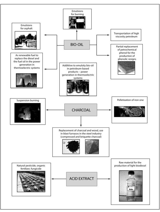
FIGURE 4 Fast pyrolysis products and its potential applications.
