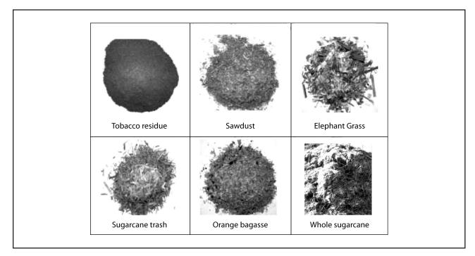
FIGURE 2 Raw materials processed at FEAGRI-UNICAMP pyrolysis pilot plant.
