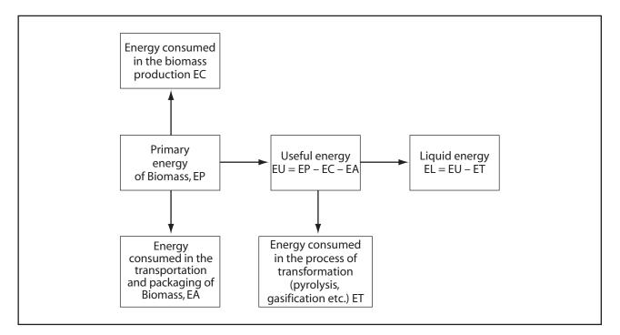
FIGURE 3 Diagram of the primary energy consumption in the productive chain of biomass transformation.
